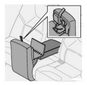
Fold the armrest in the backrest forward. Fold out the table so that it rests on the armrest. Press to release the cup holder. You do not have to fold the backrest forward, if you only want to use the cup holder.
